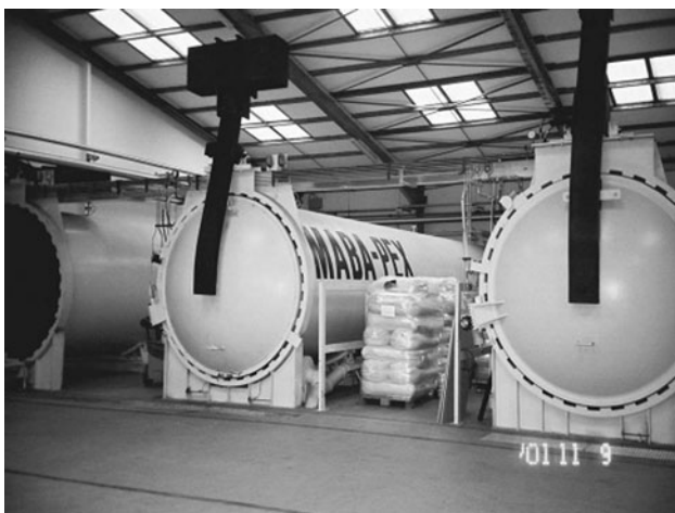
Fig. 15 Application of high pressure CO 2 for the dry fruit industry in Turkey
