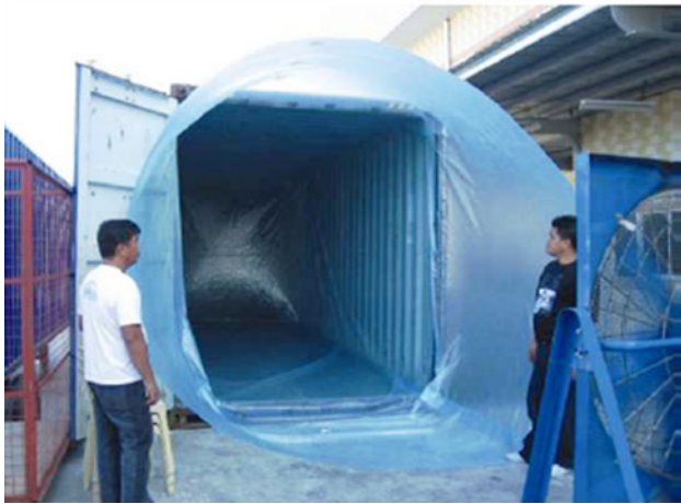
Fig. 13 TranSafeliner™ being installed in a standard shipping container (GrainPro 2008)
