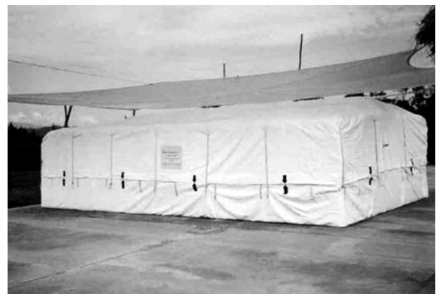
Fig. 9 Hermetic storage of corn in 150 tonnes Cocoon TM , Rwanda
